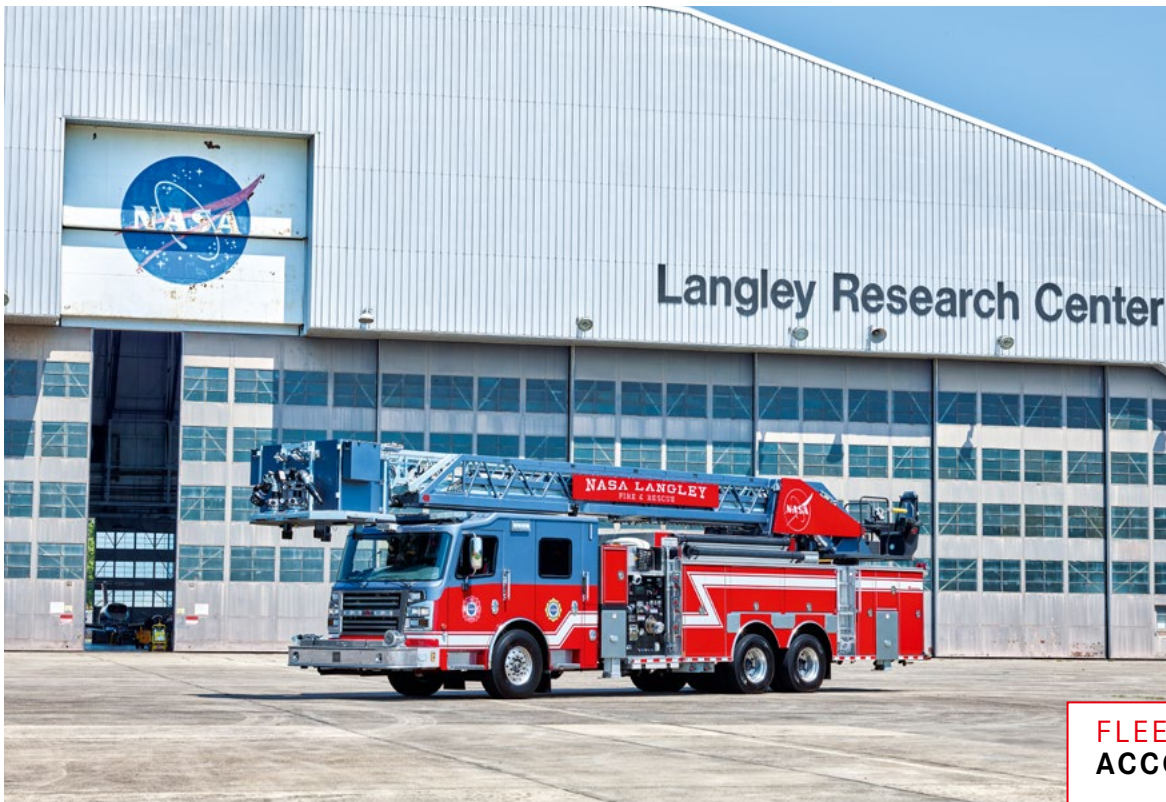
Cobra aerial rescue platform with pump and tank on Commander chassis for NASA's Langley Research Center in Virginia
