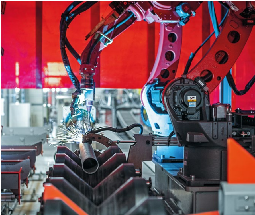
Robotized prefabrication of sprinkler pipes
