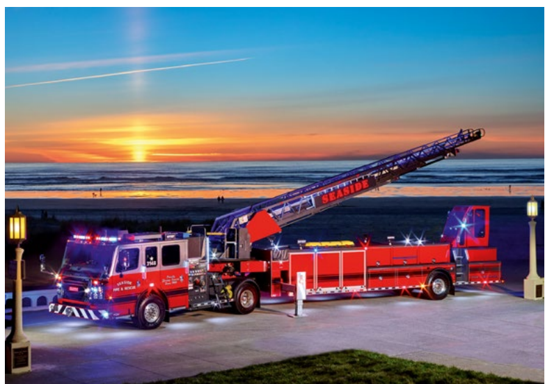
Tractor drawn aerial (tiller ladder) with steerable rear axle and 30.5 m ladder set for Seaside Fire & Rescue Department in Oregon
