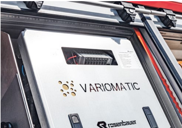
Innovative pressurized foam proportioning system Variomatic for fluorine-free extinguishing agents
