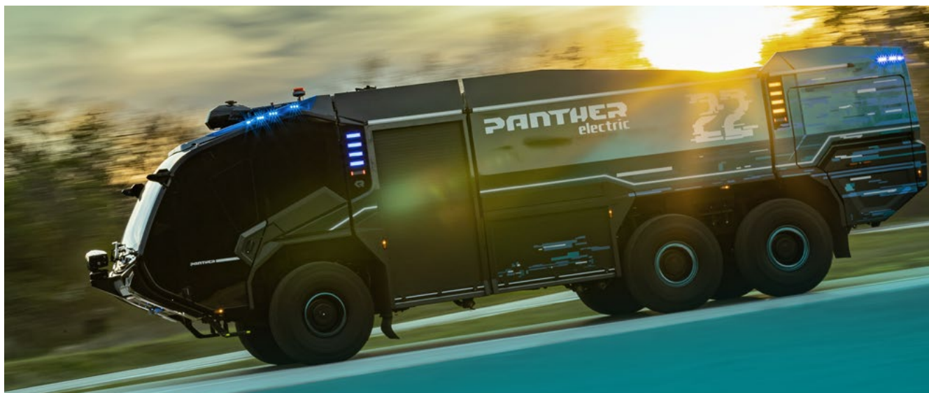
PANTHER electric: ARFF vehicle with electric drive train.
