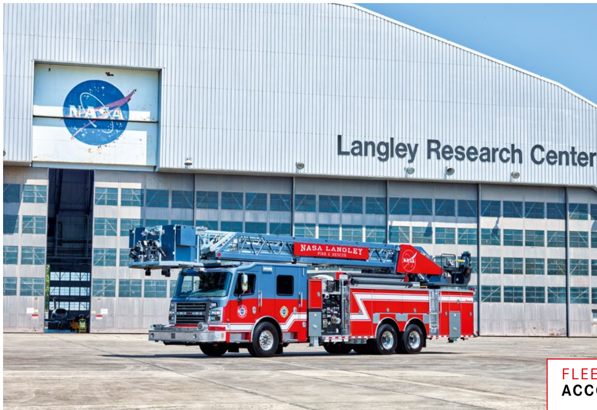
Cobra aerial rescue platform with pump and tank on Commander chassis for NASA's Langley Research Center in Virginia
