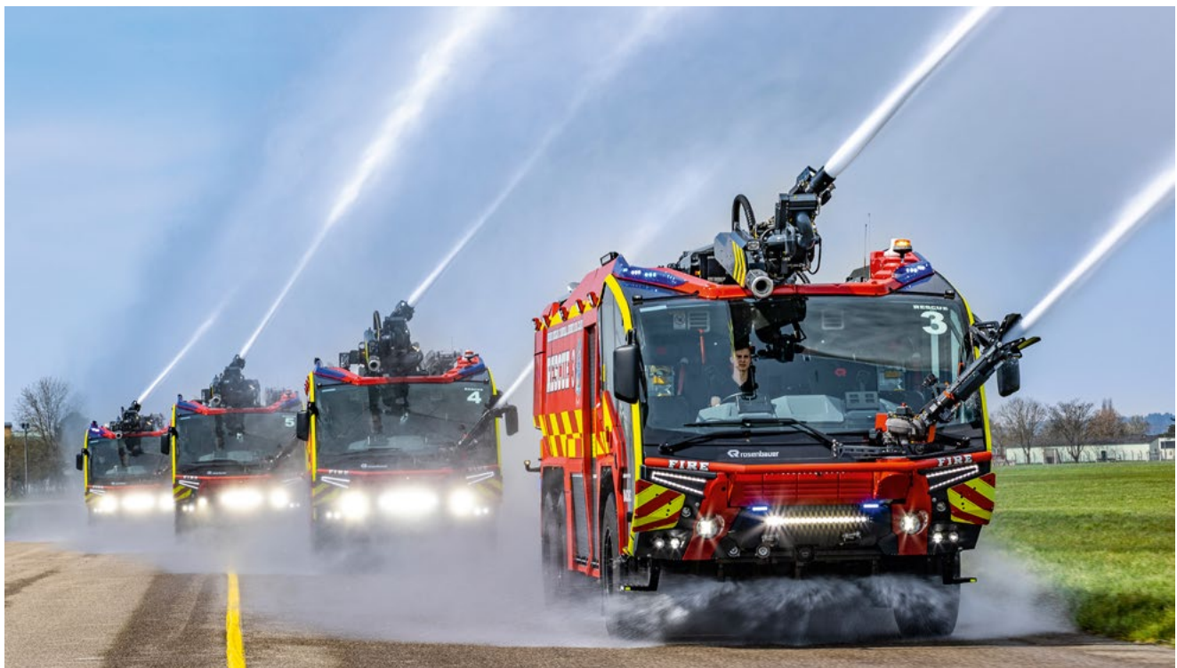
The largest water consumption in production occurs during the functional test of the turret
